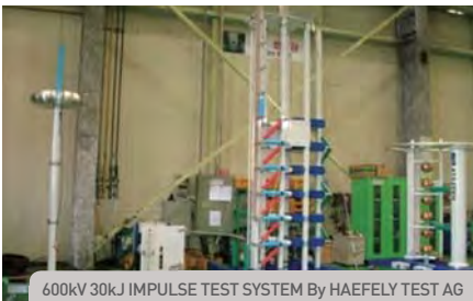
600kV 30kJ IMPULSE TEST SYSTEM By HAEFELY TEST AG
